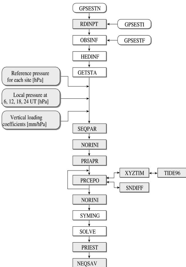
Fig. 1: Generalized flow chart of the Bernese adjustment program GPSEST; modified modules and new data files are underlined in grey.
