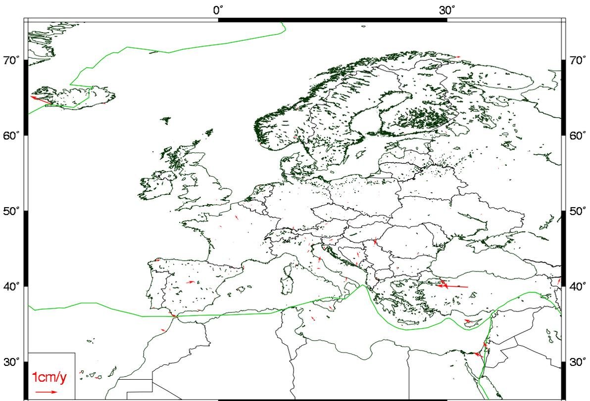
Figure 5. ETRF2000 horizontal velocities of EPN stations.
