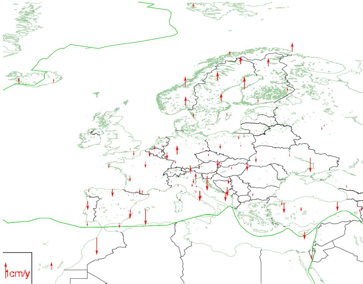
Figure 6. ITRF2000/ETRF2000 vertical velocities of EPN stations.
