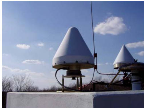
Fig. 3 – Astech choke-ring (GOPE station, left) and Topcon antennas
