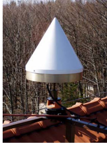
Fig. 2 – Topcon CR3 GGD antenna on metallic barrier
