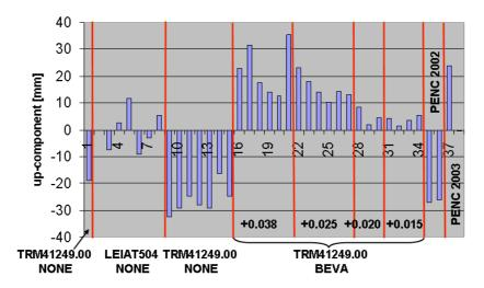
Fig. 6. Differences between TRM41249.00 antennas with radom BEVA and without to LEIAT504 antennas. Variations when the antenna height within the BEVA radom changes. Changes of PENC-WIEB after the jump of PENC (2003). Always phase corrections IGS/NGS used.
