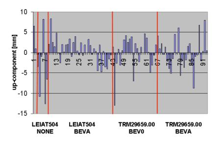
Fig. 5. Differences between TRM29659.00 with radoms BEVA/BEV0 and LEIAT504 antennas.
