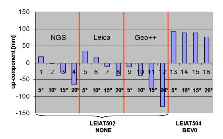
Fig. 9. Differences between LEIAT502 antennas and LEIAT504 antennas. Different phase correction sets of NGS, Leica and Geo++ are used.
