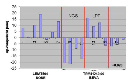
Fig. 7. Differences between TRM41249.00 antennas with radom BEVA and different phase corrections and LEIAT504 antennas.
