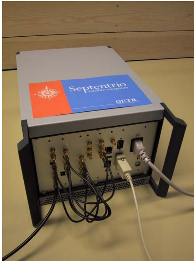
Figure 5. Septentrio's GSTB-V2 test receiver in the lab
