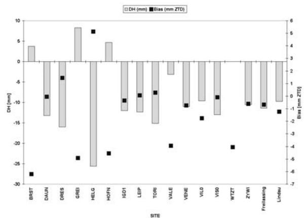
Fig. 5: Differences of ZTD and ellipsoidal height parameters: solution with coordinates fixed (to a priori coordinates) minus solution with simultaneous coordinate estimation (WTZT fixed)
