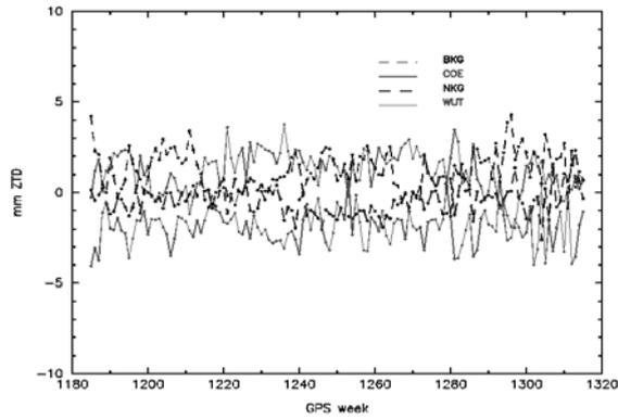
Fig. 9: Weekly mean biases for site HOFN from EPN combined solution for the four involved Local Analysis Centres
