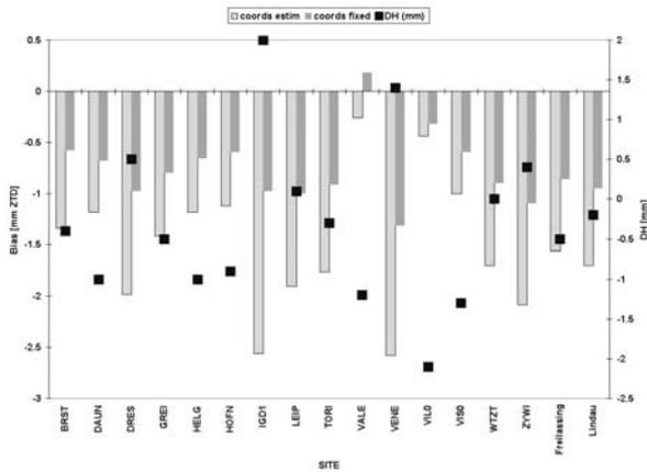
Fig. 3: Differences of ZTD and ellipsoidal height parameters: solution with (a priori/estimated) DRY NIELL/WET NIELL minus NONE/DRY NIELL; left columns and squares from analyses with simultaneous coordinate estimation (WTZT fixed), right columns from analyses with coordinates fixed to same set of coordinates
