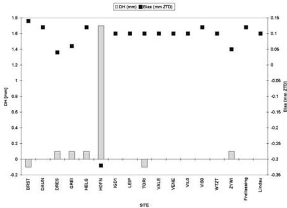
Fig. 6: Differences of ZTD and ellipsoidal height parameters: solution with consistent Ocean Tide Loading (OTL) parameter set minus OTL parameters changed for station HOFN (WZTJ fixed)
