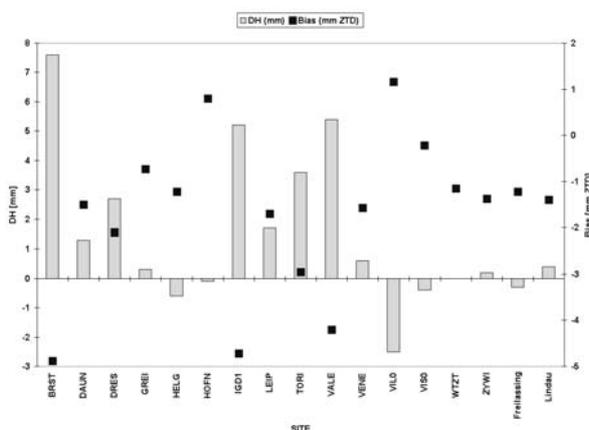
Fig. 4: Differences of ZTD and ellipsoidal height parameters: solution with estimation of horizontal gradient parameters (TILTING) minus solution without horizontal gradient parameters (WTZT fixed)
