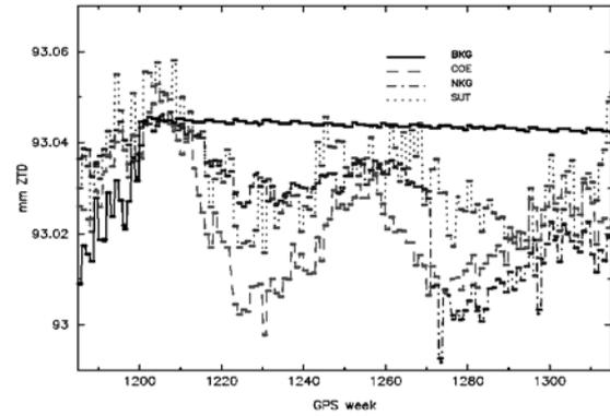
Fig. 12: Estimated ellipsoidal height for site REYK taken from combined weekly SNX files
