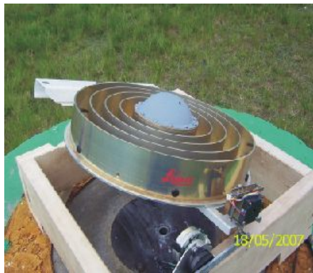
Fig. 2. Investigation of the Leica choke-ring antenna before its installation at the permanent GPS station LAMA
