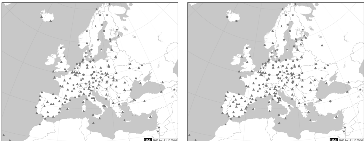
Figure 6 – Left: Antenna/radome calibrations used within the EPN in Dec. 2006, Right: Antenna/radome calibrations used within the EPN in June 2008 (circle: individual absolute robot calibrations; triangle: type absolute robot calibrations; square: absolute calibrations converted from relative field calibrations, star: no absolute calibrations available).
