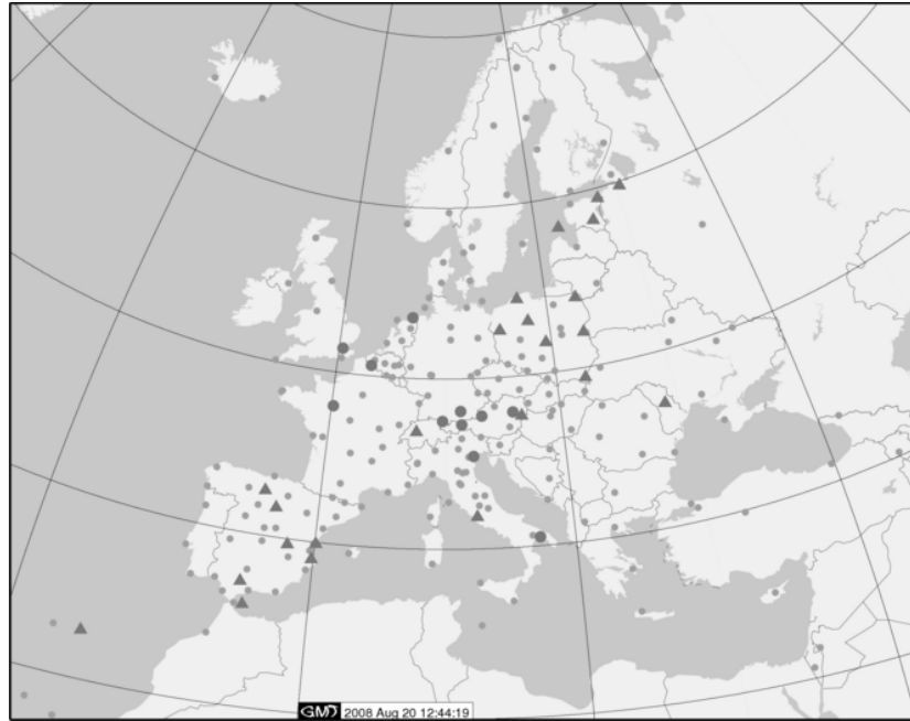
Figure 1 – EUREF permanent tracking network (status June 2008); triangles: the stations added to the network since June 2007; circles: stations removed from the network since June 2007.
