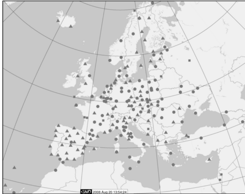
Figure 3 – EPN stations classified following data flow. Triangles: stations streaming data in real-time; Circles: stations making available hourly data and squares: stations make available daily data only.
