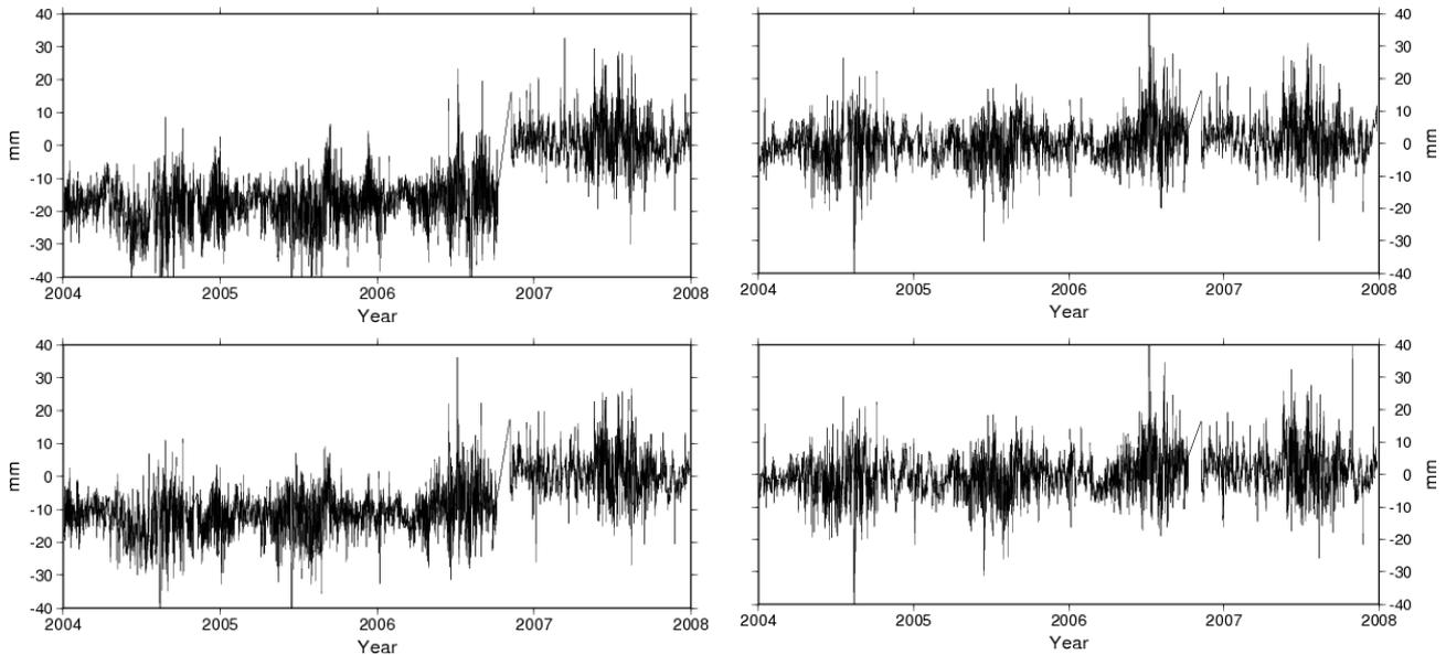
Figure 4: Time series of ZTD differences between radiosonde and EPN combined solution (left) as well as MUT reprocessing solution (right) for site Borowa Gora, Poland, with co-located stations BOGI (upper part) and BOGO (lower part).
