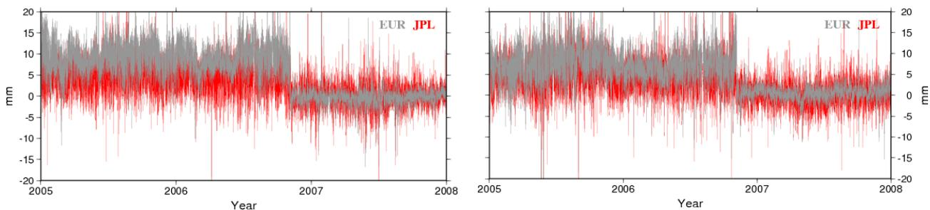
Figure 2: ZTD differences between MUT solution and EPN combined solution (in gray) and IGS PPP solution (in red) for the stations BOR1 (left) and SFER (right).
