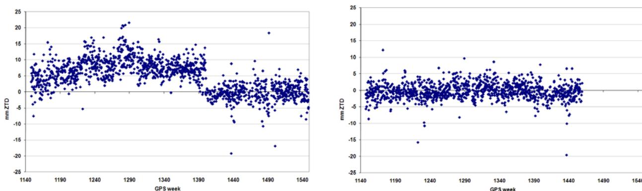
Figure 3: Daily ZTD biases between IVS combined solution and EPN combined solution (left) as well as MUT solution (right) for site Wettzell.
