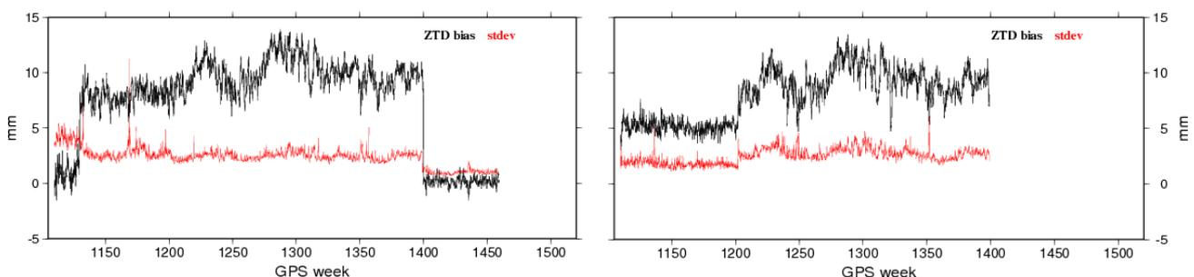
Figure 1: Weekly mean ZTD bias and its standard deviation between MUT reprocessed solution and EPN combined solution (on the left) and IGS combined solution (on the right). Note that a) IGS combination stopped with GPS week 1399 and b) EPN combined solution contributed to IGS combination since GPS week 1203.
