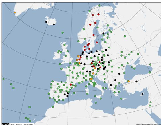
**Fig. 4:** Overview of the absolute receiver antenna calibrations used in the EPN analysis. Left: using epn\_05.atx, right using epn\_08.atx. Black: individual calibrations, green: robot calibrations, orange: from field/relative calibrations, red: uncalibrated radome. The circles indicate regions where a clear improvement is seen.
