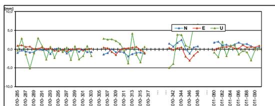
**Figure 9.** Station KATO - equipment exchange (17-12-2010). Trimble NETRS with TRM41249.00 TZGD antenna replaced by Trimble NETR5 with TRM57971.00 TZGD antenna
