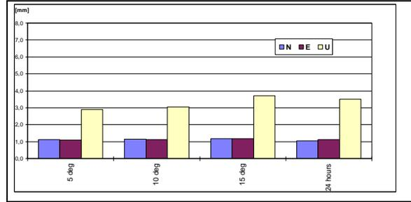
**Figure 5.** Daily repeatability of co-ordinates for different type of processing determined for 2008 campaign
