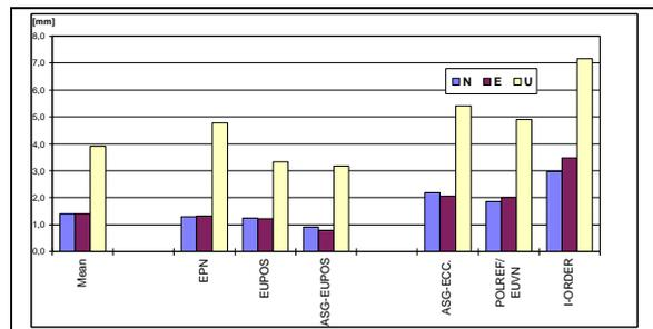
**Figure 7.** Daily repeatability of co-ordinates determined for different type of measured stations for 2010/2011 campaign.
