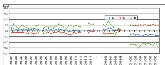
**Figure 10.** Station WODZ - equipment exchange (09-02-2011). Ashtech UZ-12 with ASH701945C M SNOW antenna replaced by Trimble NETR5 with TRM57971.00 TZGD antenna
