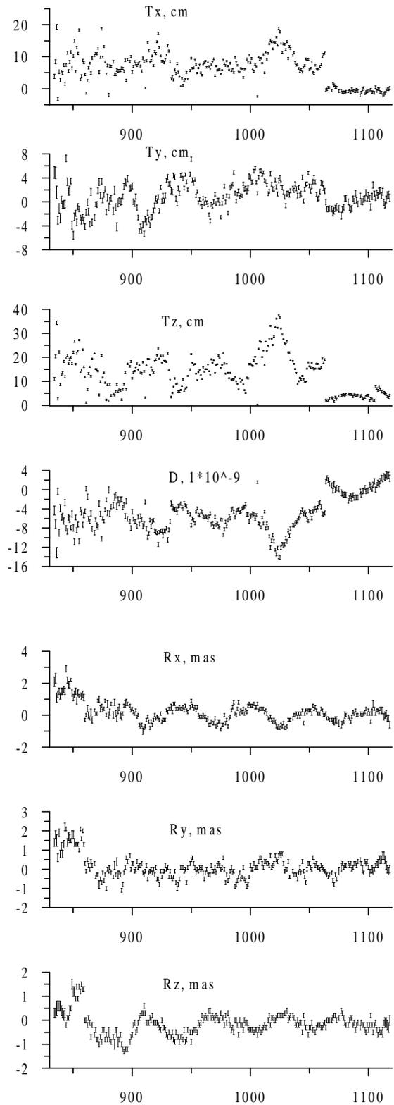
**Fig. 2** Time series of parameters for 7-parameter transformation between free weekly solutions and ITRF2000 (R – rotation parameters, T – translation parameters, D–scale parameter).
