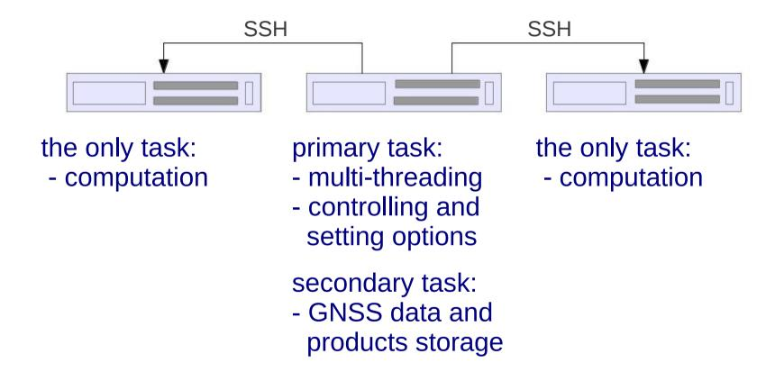
Type of all the three machines: Asus RS120-E4PA2, Intel Xeon X3220 2.4Ghz, 4GB DDR2800, 2x250GB WD 7200rpm RAID1
