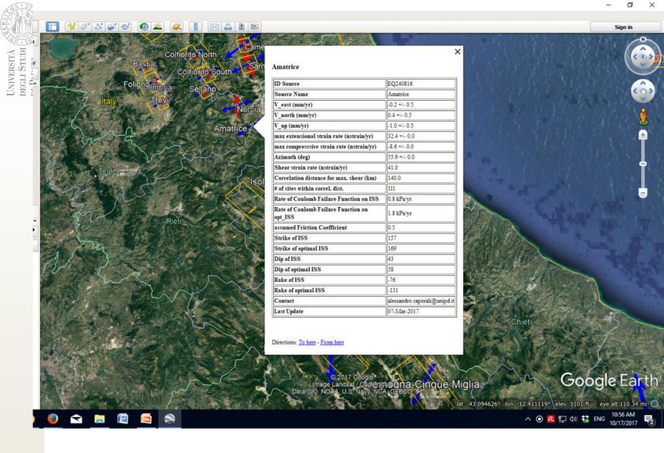
Strain rates and Coulomb loading rates are computed at the Individual Seismogenic Sources catalogued by INGV (light brown rectangles)
