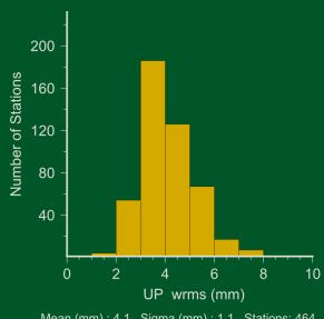
Mean (mm) : 4.1 Sigma (mm) : 1.1 Stations: 464 50% < 3.9 (mm) 70% < 4.4 (mm) 95% < 6.0 (mm
