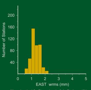
Mean (mm) : 1.3 Sigma (mm) : 0.4 Stations: 464 50% < 1.3 (mm) 70% < 1.4 (mm) 95% < 1.9 (mm
