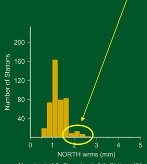
Mean (mm): 1.3 Sigma (mm): 0.4 Stations: 464 50% < 1.2 (mm) 70% < 1.4 (mm) 95% < 2.1 (mm)
