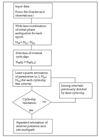
Fig.1 – Flow chart of PERMGPS-QC software
