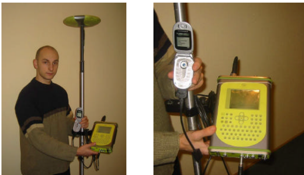
Fig. 19. A set of surveying instruments implemented for EUREF-IP RTK survey
