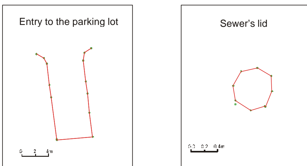
Fig. 17. RTK Ntrip survey of some municipal features
