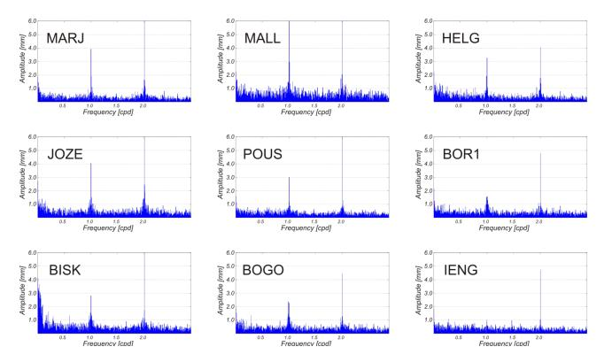
Fig. 3 Periodograms of sites with oscillations in height component (amplitude higher than 3 mm).
