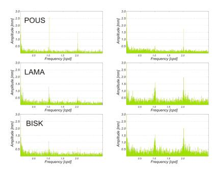
**Fig. 6** Periodograms of sites with oscillations in horizontal components (amplitude more than 1 mm), left: N-S component, right: E-W component.
