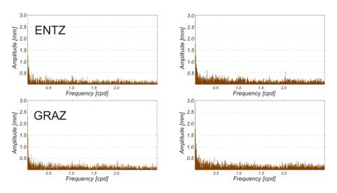
Similarly to height the horizontal components were divided into two groups. 1 mm was taken as the threshold. Most of stations with oscillations below 1 mm are located in Central/Western Europe.
